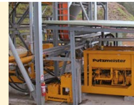
HSP 25100 HPS, PCF-Ventile, Hydraulikaggregat HA 400 + 400 E-SP
